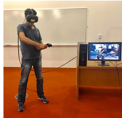
Figure 1—Virtual Reality experience: The headset’s cable not only limits the player’s mobility, but also creates a tripping hazard.
